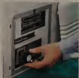
Remove the right hand quick access panel to uncover the RAM, cache and CPU.
